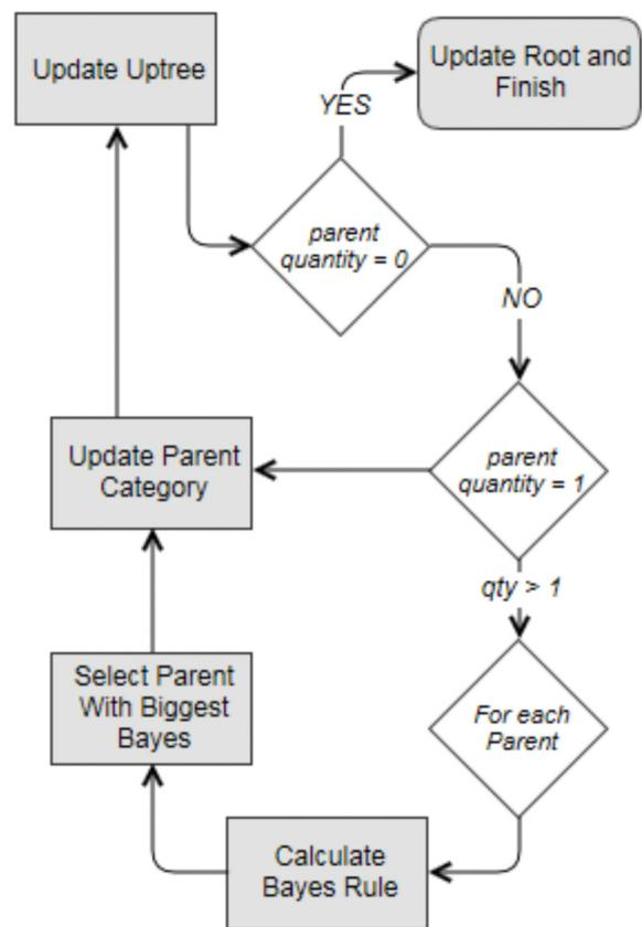
Fig. 9. Second part of the distribution algorithm's pseudocode: update up-tree.
