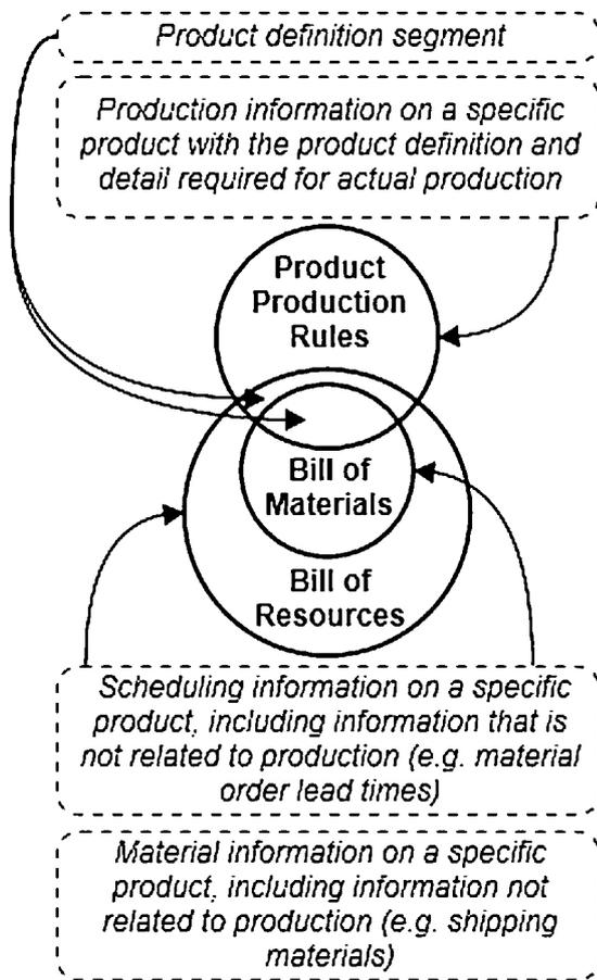
Fig. 2. Overlay chart for the *Production Definition* category, on the Part I of ANSI/ISA-95 standard.
